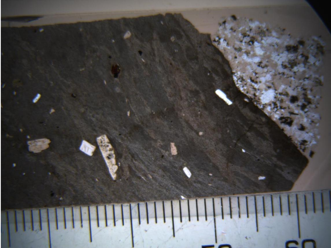
Figure 5: Photomicrograph of GR2 in PPL, showing sharp boundary between lithic and host rock, as well as cooling fractures. Shows rounded edge.
