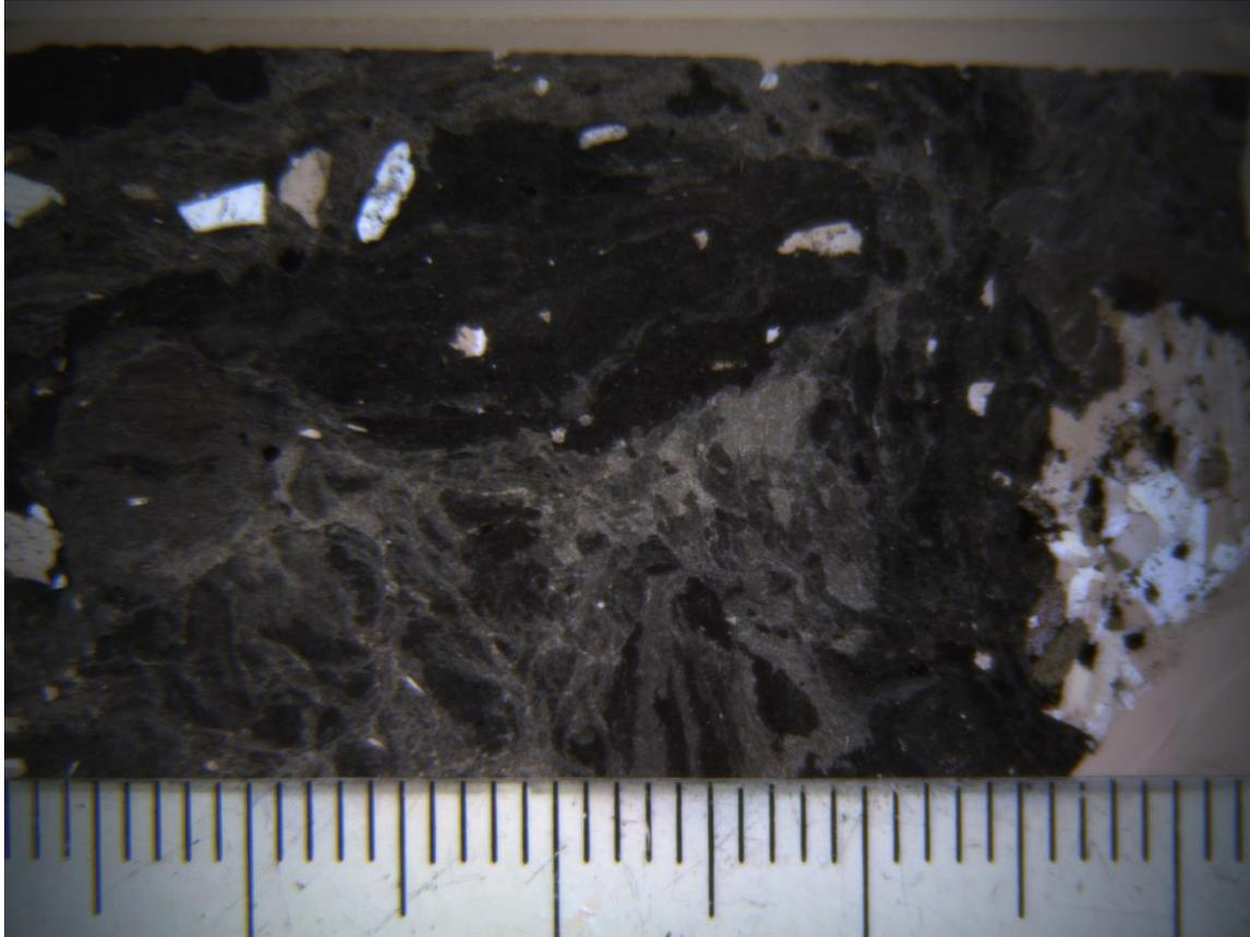
Figure 6: Photomicrograph of GR8 showing the sharp jagged boundary between lithic and the host rock
