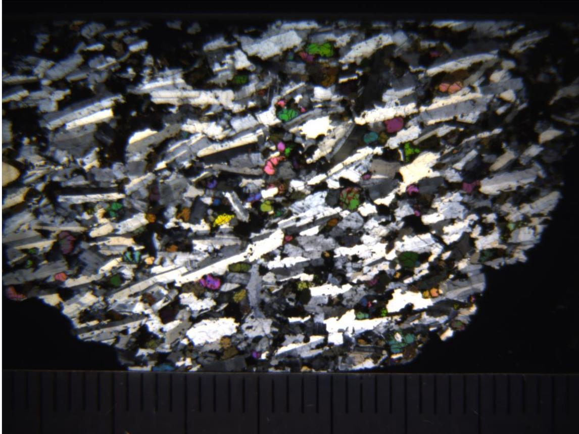
Figure 7: Photomicrograph of GR17 in XPL, showing alignment of feldspar crystals
