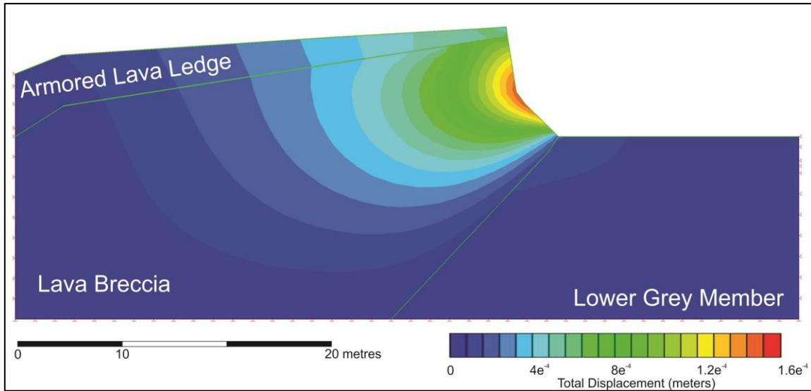
**Figure 3.** Stability model of the outlet created using Phase2 by Rocscience. This model reflects the outlet under static conditions.
