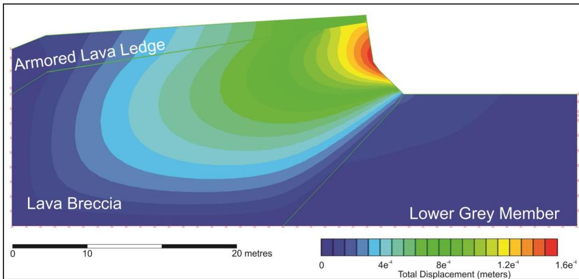
**Figure 4.** Seismic loading model with a PGA of 0.3g applied.
