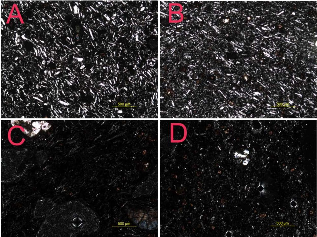
**FIGURE 3** Thin sections taken along the length of the flow from both the rubbly and massive portions of the flow showing the increase of groundmass crystallinity. (A) and (B) are from the massive part of the flow, (B) is sourced 30 meters down-flow from (A) and shows an increased crystal density. (D) is sourced 30 meters down-flow from (C) and also shows an increase in crystal density
