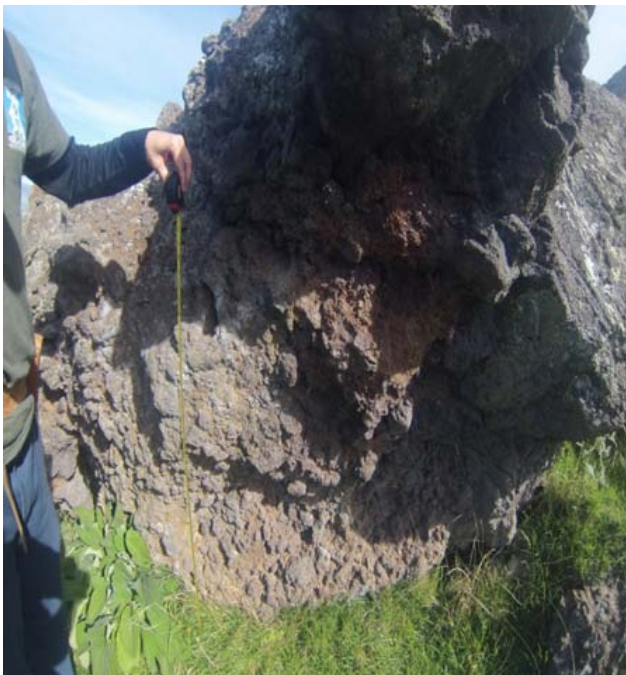
245 *Figure 3: Photo taken of RAP #03 Section 2 prior to clast count (left) compared with same 246 photo after 1m 2 grid is drawn in and clasts have been colored black in Microsoft Paint for pixel 247 counting.
