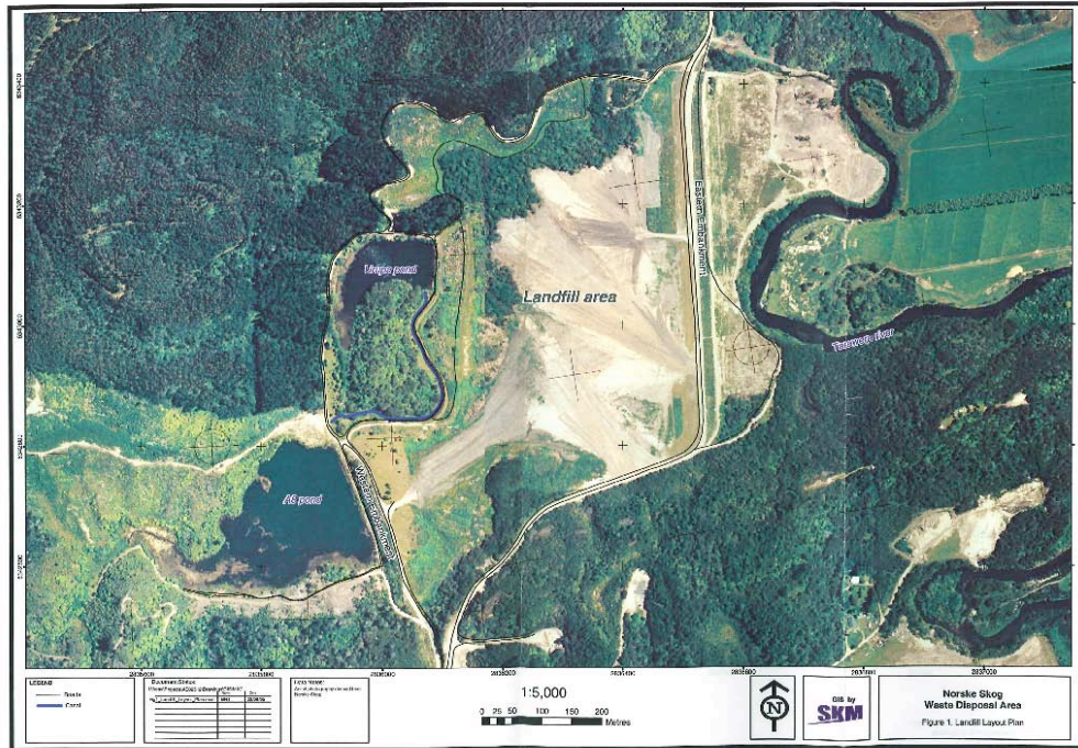
Figure 4: The waste disposal site of the Tasman Pulp and Paper Mill in the land leased from the Ngati Tūwharetoa ki Kawerau tribe, showing Lake Rotoitipaku filled in with solid waste.
