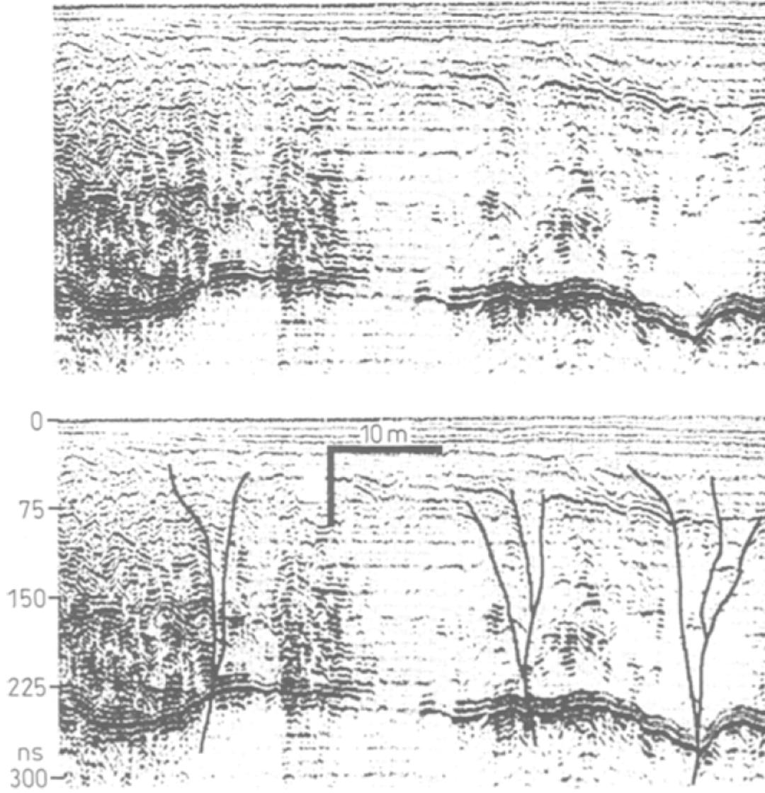
**Figure 6.** Example of GPR interpretation taken from Wyatt and Temples (1996). This figure showcases the subjectivity of GPR profile interpretation in the presence of broken reflectors. The middle fault structure may be discernible, but the two on the outside could arguably be drawn on different lines.
