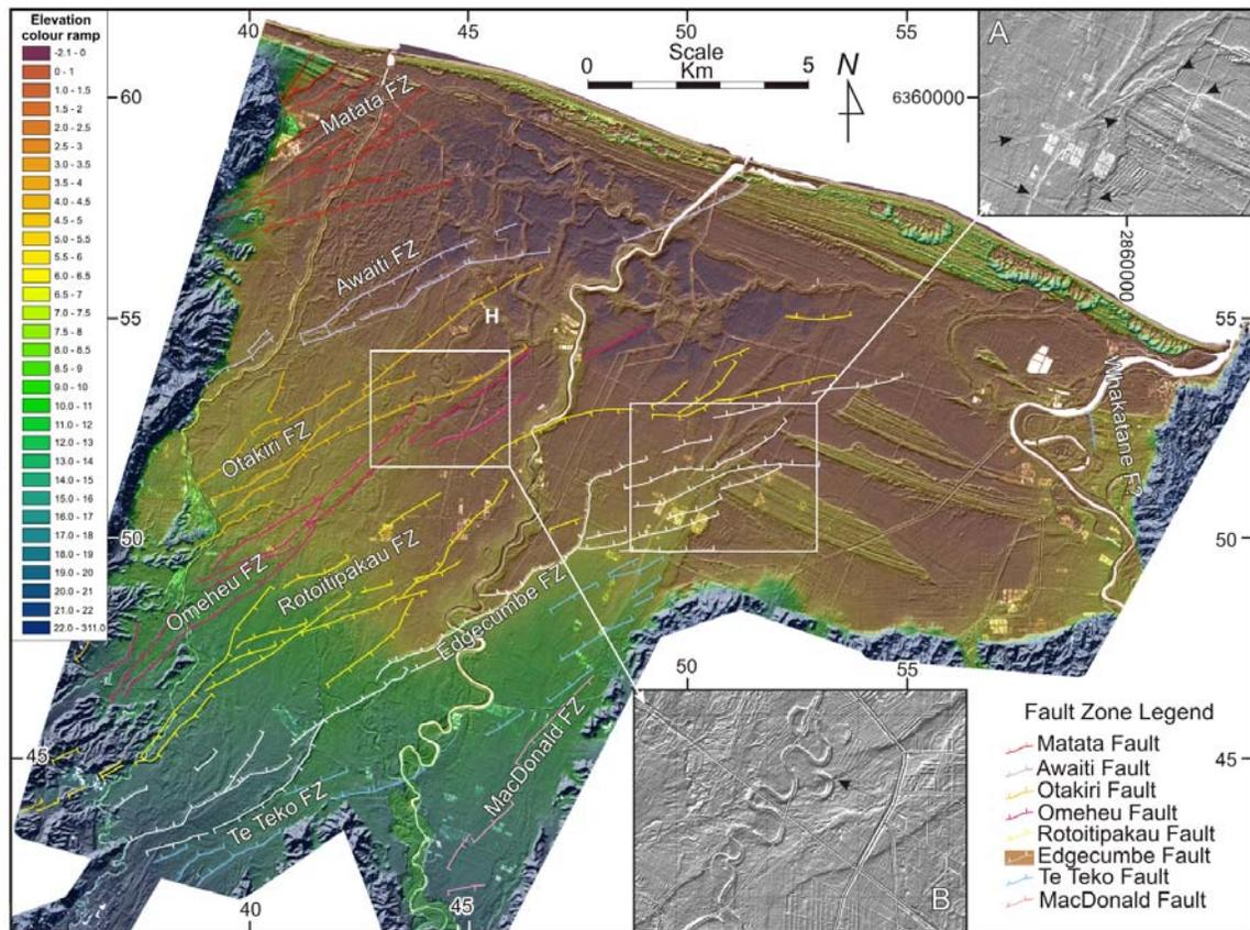
**Figure 1.** LiDAR data map of newly found faults in the Whakatane Graben. Image is as presented by Begg and Mousopoulou (accepted). The series of faults explored in this study are contained in the white box on the right.
