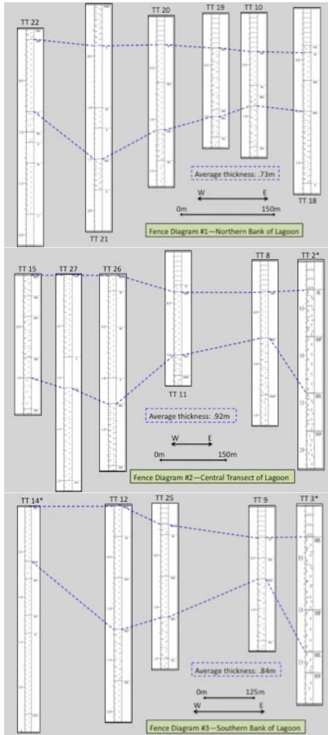
borelogs from the northern transect were re-examined for the clay layer. As anticipated, two of the six logs contained a silt layer with plant remnants atop the debris layer material—concluded to be the ambiguous clay layer seen in the GPR reading (Dougherty 2010 pers. comm.).
