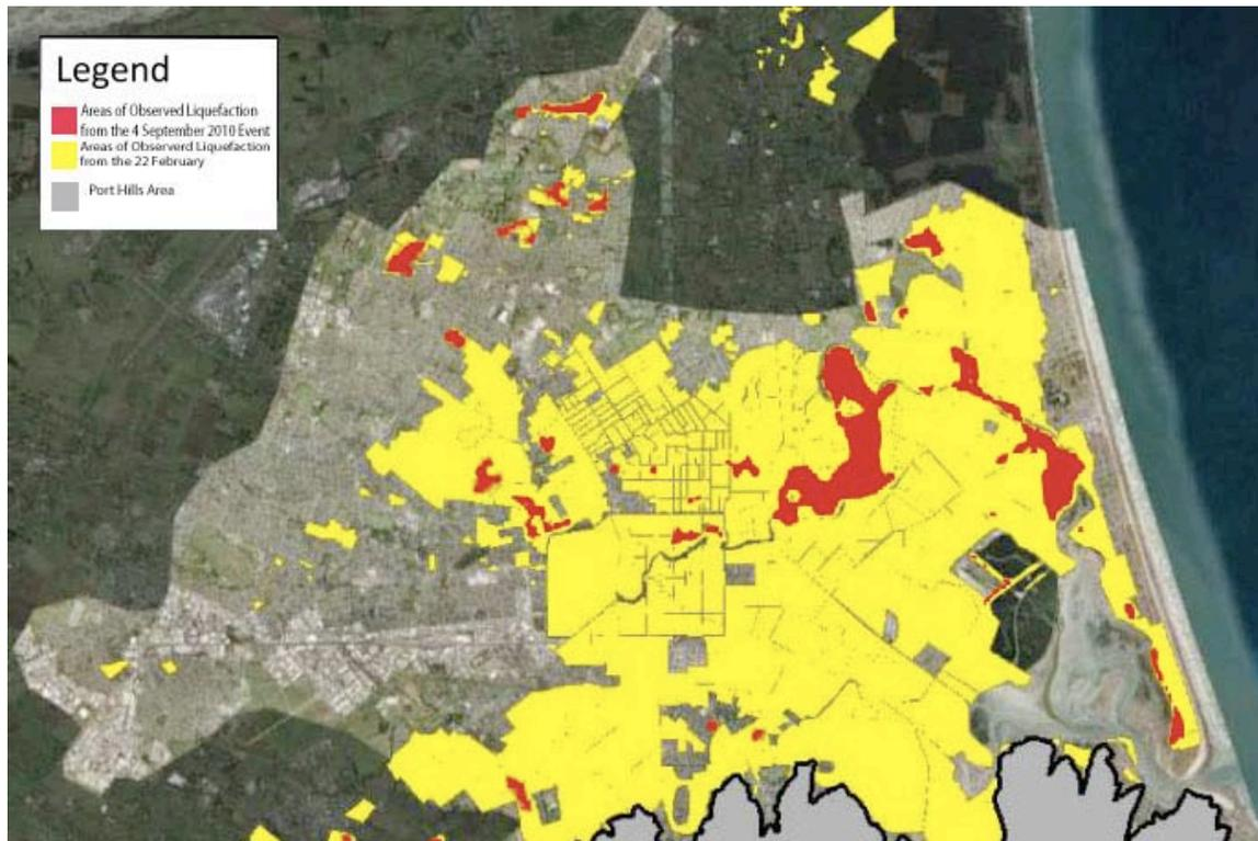
Figure 1 Areas of liquefaction damage in Christchurch from the September 2010 and February 2011 earthquakes. Adapted from the Canterbury Earthquake Recovery Authority
