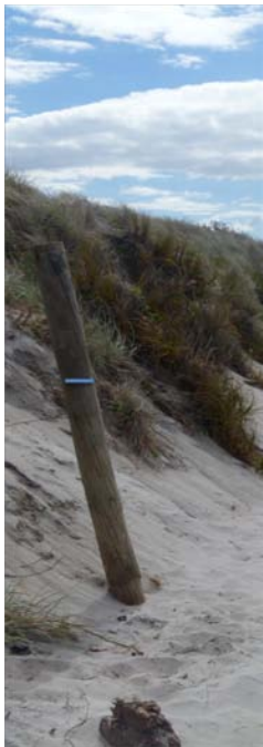
Figure 5.1. Line indicating position at which above it the pole was wet and below it the pole was dry.
